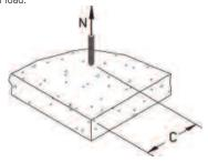
1/4 3/8 1/2 Dia. (in.) 3/16 C<sub>cr</sub> (in.) 2 5/8 3 1/2 5 1/4 C<sub>min</sub> (in.) 1 1/4 1 7/8 2 1/2 0.25 1 1/4 0.25 Edge Distance, c (inches) 1 7/8 0.67 0.46 0.25 0.72 0.50 0.28 2 1/2 0.94 0.67 0.39 0.25 2 5/8 1.00 0.71 0.42 0.27 3 3 1/2 0.83 0.50 0.33 1.00 0.61 0.42 4 0.50 0.72 5 1/4 0.94 0.67
